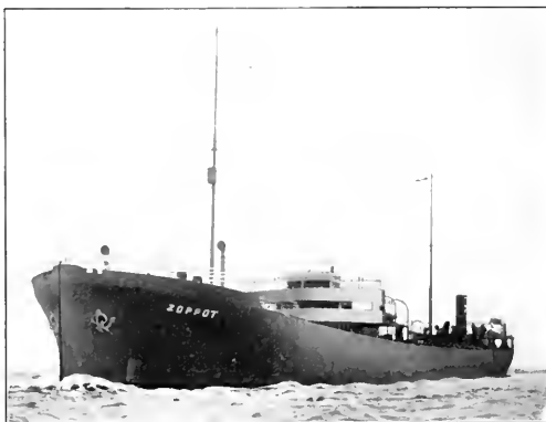
THE MOTOR TANKER ZOPPOT Length over all 546.91 ft., 9,932 Gross Tons, Cargo Capacity 5,186,774 gallons, speed 10.5 knots, equipped with two 1,700 B. H. P., two cycle, six cylinder KRUPP DIESEL ENGINES.
